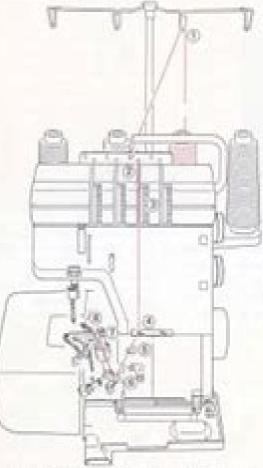
Place the speel of thread on the speel pin second from the right.
