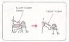
Turn, the balance wheel toward you until the upper looper comes to the middle point of its travel, and unbook the thread of the lower looper from the upper Isoper.
