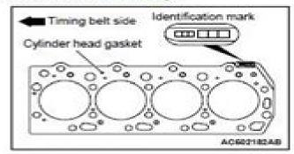
When replacing the cylinder head gasket only, confirm the gasket identification mark, and then select a replacement part according to the following table.
