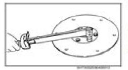
TIGHTEN THE FLEX PLATE, SPACER COUPLING AND WEAR PLATE.
