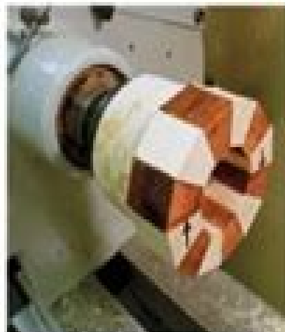
Figure 3-38: Blank mounted to the waste block with hot glue and smooth ends.
