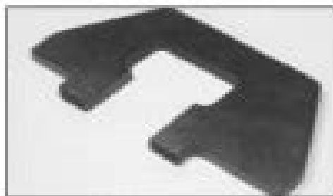
10.11a The BMW tool for holding the camshaft in the TDC position on M40 engines
