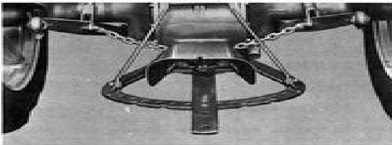
Fig. 8 - Swinging Drawbar with PTO Adapter Installed
