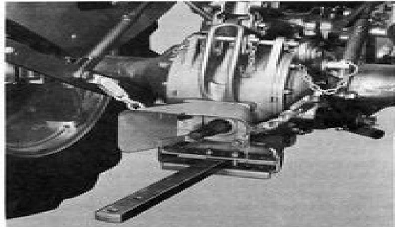
Fig. 9 - Universal Drawbar with PTO Adapter Installed
